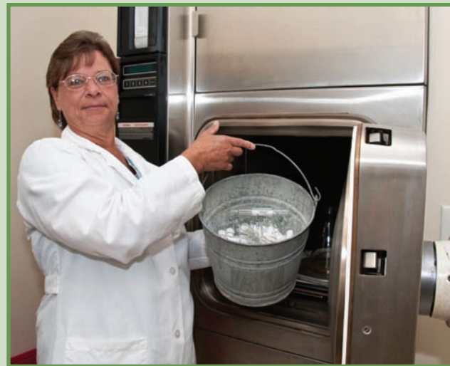
Diane Suhocki removing a bucket full of sterilized glass culture tubes from the autoclave.
